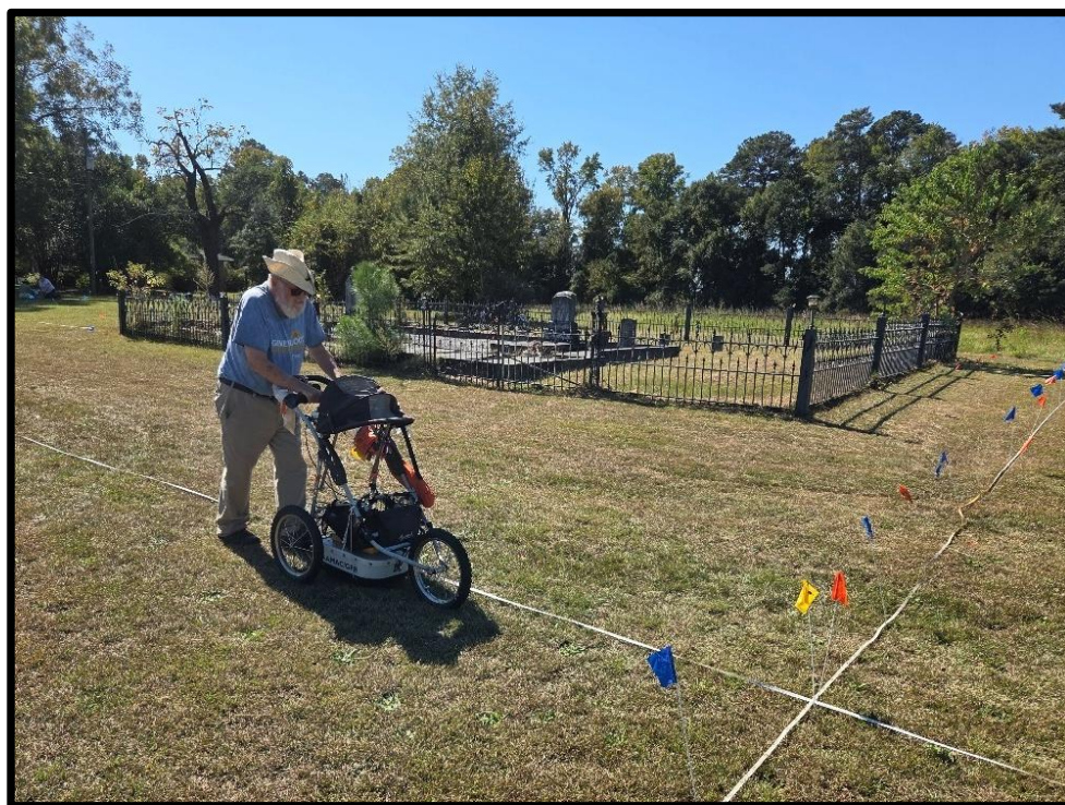
Figure 36. Ground-Penetrating Radar in use outside the McCoy-Mathews-Ryals Burial Ground, courtesy SAH
